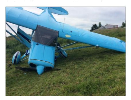
**Photo No. 2**: Damage to undercarriage, wing, cowling and propeller.
